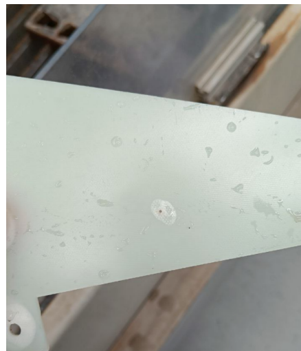
Figure 3.1.5.3.2: Delamination in fiberglass from waterjet using the low-pressure setting.
