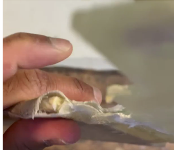
Figure 3.1.5.4.4: Fiberglass Overlay Separation
