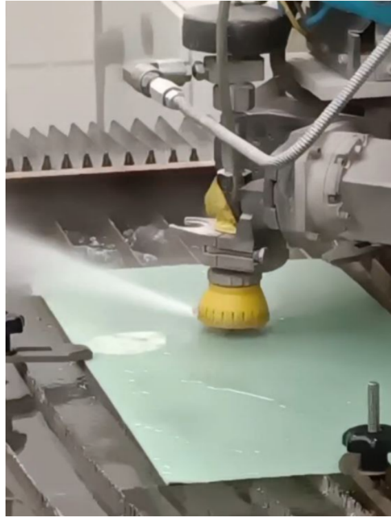
Figure 3.1.5.3.3: Anomaly in the operation of waterjet cutting. The water jet reflects from the fiberglass sheet.
