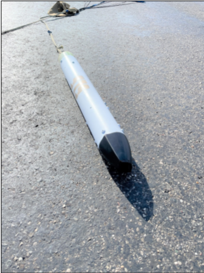
Figure 3.3.2.1b: Nose cone and upper stage. Image has been brightened to show deformation in the nose cone upon landing.
